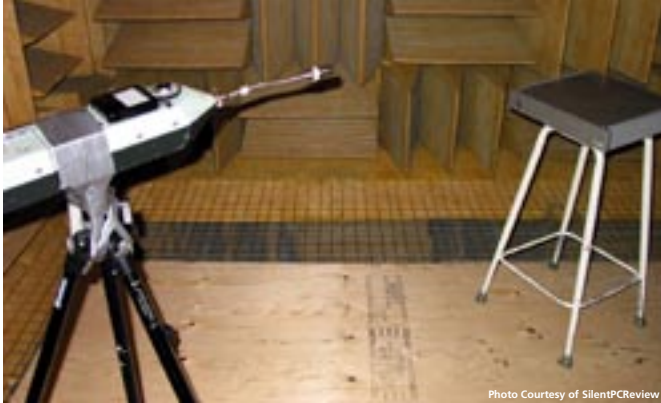
A sound level meter in an anechoic chamber
