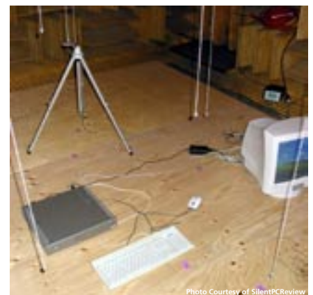
An anechoic chamber used for sound power readings
