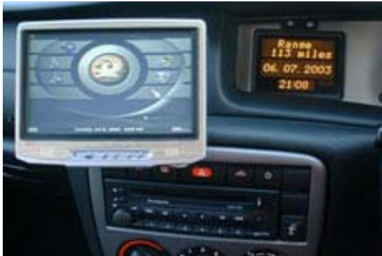
“Vauxhall Vectra CarPC Project” VIA EPIA 800 board with Digitalww touch screen, a Opus intelligent ITX DC to DC PSU
